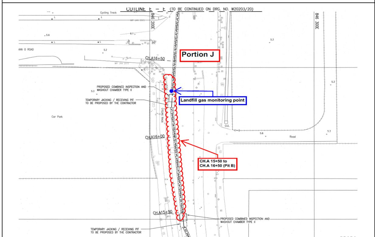
Figure 4.4 Monitoring Location – CH.A 15+50 ~ 16+50 (Jacking Pit B)
